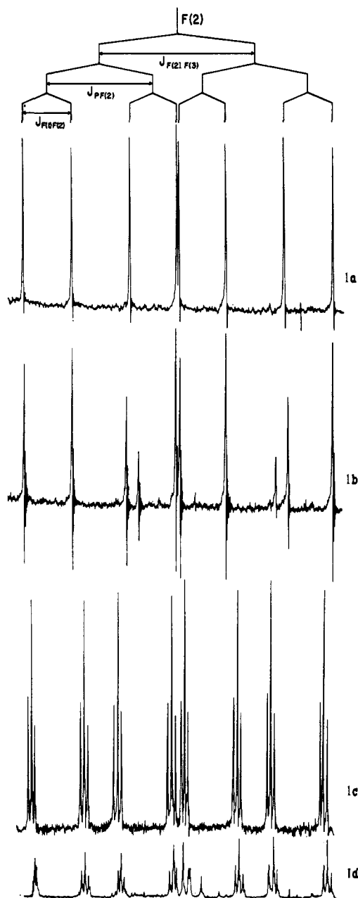
Figure 1. (a) ^{19}\text{F} nmr spectrum of F(2) of \text{CF}_2=\text{CFPCl}_2 phase detected undecoupled. (b) ^{19}\text{F} nmr spectrum of F(2) of \text{CF}_2=\text{CFPCl}_2 with lowest field line of F(3) irradiated at 5012 Hz. (c) ^{19}\text{F} nmr spectrum of F(2) of \text{CF}_2=\text{CFPF}_2 phase detected undecoupled. (d) ^{19}\text{F} nmr spectrum of F(2) of \text{CF}_2=\text{CFPF}_2 with lowest field line of F(3) irradiated at 5479 Hz.
